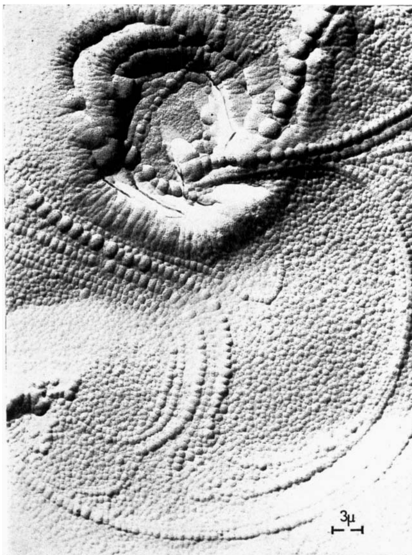
Figure 4. Electron micrograph of a replica of quench-frozen neat phase containing 20% water. Magnification 36,000\times .
